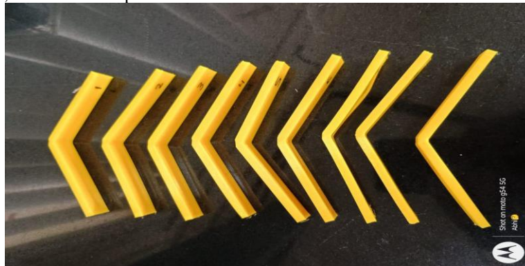
Figure 6: Flexural Specimens After Test
